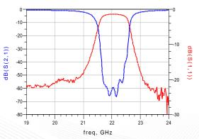
Band rejection & Return loss  $\rm VS$  frequency  $(T_A\!=\!\!25^\circ\!{\rm C\,})$
